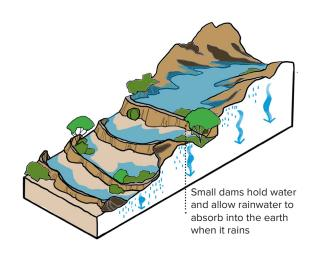
**INFILTRATION AND TREATMENT-BASED LANDSCAPES** slow overland flow, increase groundwater infiltration to recharge aquifers, manage flood risk and reduce erosion.
