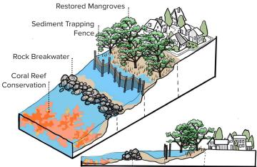
**BREAKWATERS** reduce wave energy to buffer impacts of weather events to vulnerable communities and facilitate sediment accumulation for ecosystem restoration, such as for mangroves.
