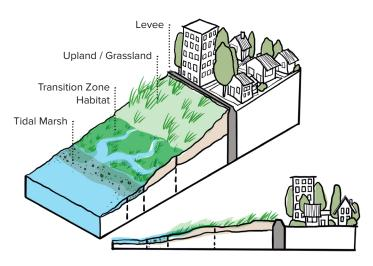
**HORIZONTAL LEVEES** integrate coastal ecosystem restoration and/or conservation with traditional levee design to achieve greater protection from floods and sea level rise than if either solution was applied alone.
