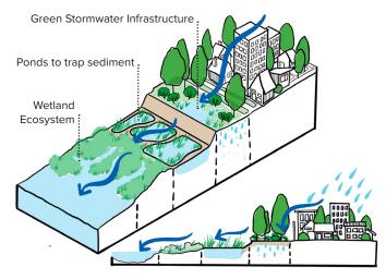
**CONSTRUCTED WETLANDS** use natural processes to clean stormwater, graywater and/or wastewater, resulting in improved habitat and biodiversity benefits. Stormwater wetlands clean runoff from urban spaces, reduce flooding and create spaces for people to access nature.
